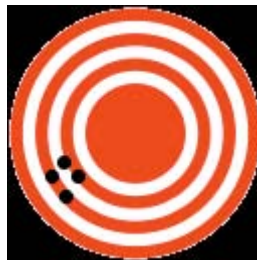
Figure 14 - High precision but low accuracy
